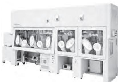
Cell Processing Isolator (CPI) - manual glove port access.
